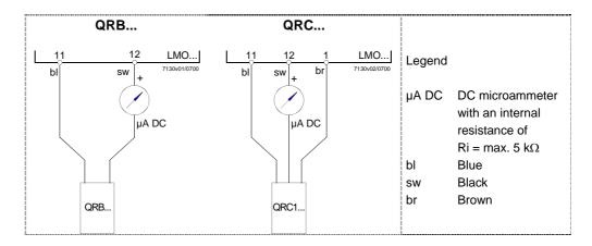
As an alternative to detector current measurement, the diagnostic tool OCI400 / ACS400 can be used. In that case, the DC microammeter is not required.
