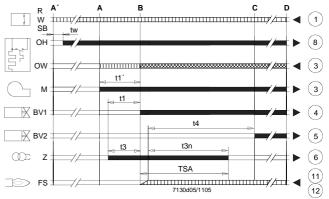
AL Alarm device BV... Fuel valve
